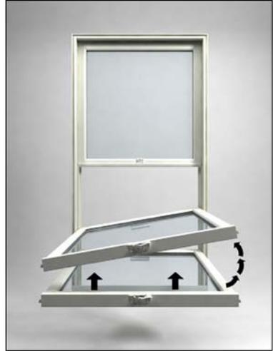
When sash is in a horizontal position, lift both sides of the sash upward 2-3" (raising pivot pins out of each clutch). Now rotate the sash until pivot pins clear the jambs and remove the bottom sash from the frame.
