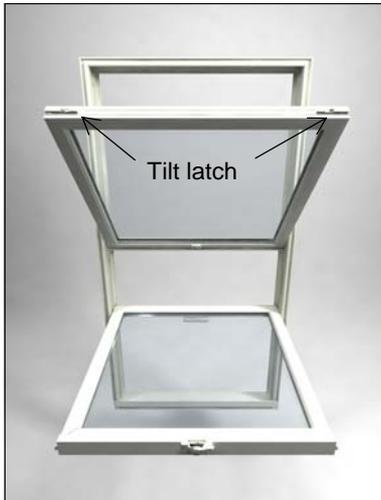
To tilt the top sash, lower the sash about half way. Pull the tilt latches inward (located on the top edge of the sash rail) simultaneously until they clear unit frame. Ease top of sash to a horizontal position.
