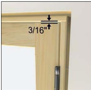
Check panel alignment with locking jamb; panel should have 3/16" clearance along the jamb. Rotate horizontal adjustment screw clockwise to increase, counterclockwise to decrease jamb/panel clearance at the appropriate hinge i.e. if increasing clearance at top, bottom hinge may have to be adjusted to decrease clearance to avoid hinge binding. See illustration.
